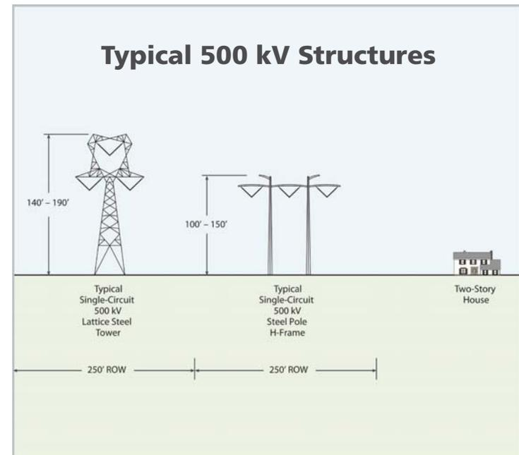
Note: Graphic of typical structure. Heights may vary due to terrain and engineering constraints. Other tower types may be used based on local circumstances.
